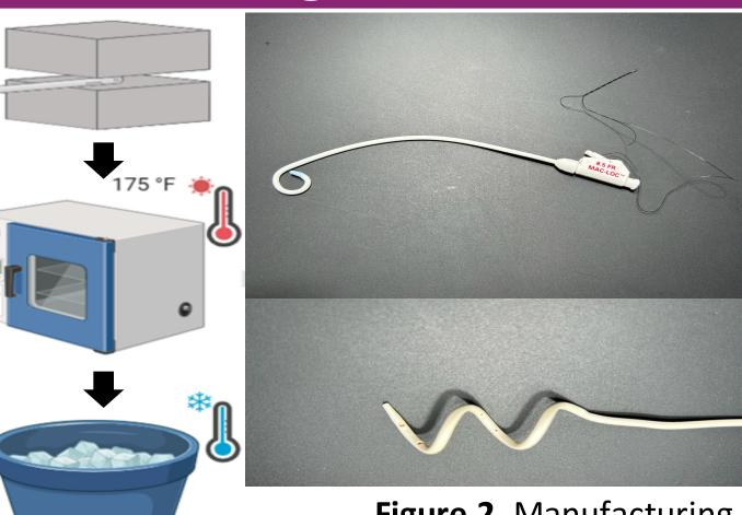
Figure 2. Manufacturing method and catheters used.
